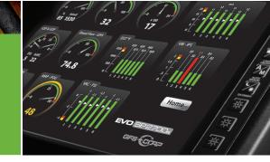
Active Display Area: 245.76 (H) x 184.32 (V) Resolution: 1024x768 Ambient Operating Temperature: -20 to 60 °C (-4 to 140 °F) Humidity: 10% to 95% non-condensing Shock: 15G, 11 ms duration Vibration: 5 Hz ~ 500 Hz / 1 Grms
